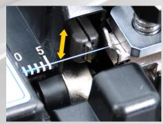
A new blade mechanism controls blade height automatically. It keeps good blade condition to obtain stable cleaving quality.
